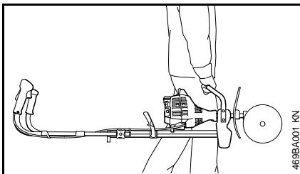
Grip the power tool by the carrying handle with the attachment facing forward.
