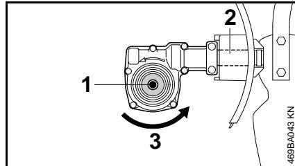
Gearbox output shaft (1) below the drive tube (2).
