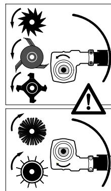
On metal tools (top illustration), position the gearbox so that the shaft is below the drive tube.
